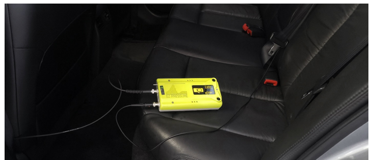
Pressure gauge placed on the back seat.
