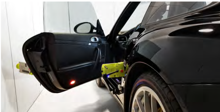
EZSlam placed on frameless car door.
